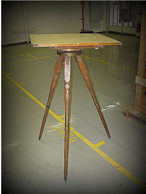
Figure 6: Original surveyor's plane table from Marinoni, Lombardia, about 1770 (Vienna Technical Museum). Most probably the officers were equipped with a pattern of this type.
